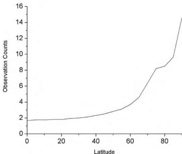
Figure 4. The average overpass counts of MODIS from both Terra and Aqua satellites over a time period of 12 hours as the function of latitude.
