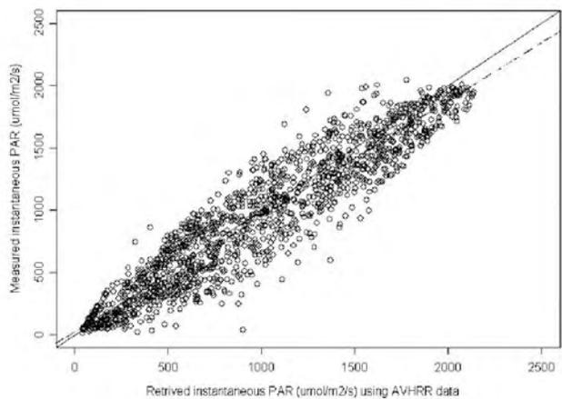
Figure 3. Validation of the AVHRR-derived instantaneous PAR data at the three FLUXNET sites. The solid line is the 1:1 line and the dashed line is the best fit line based on least squares regression. Table 1 provides the statistics for the best fit line.
