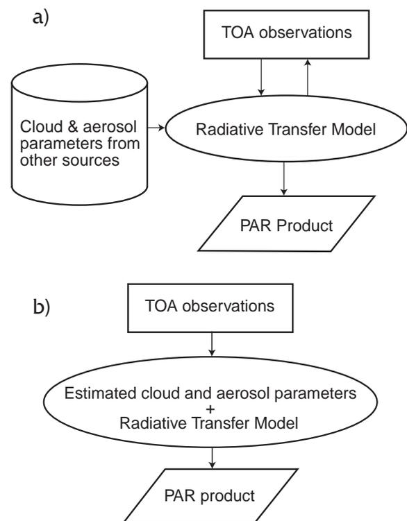
Figure 1. Illustration of two methods for estimating incident PAR from satellite observations.
