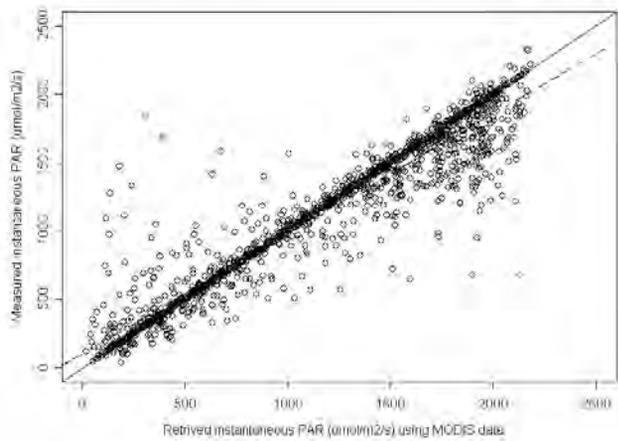
Figure 2. Validation of MODIS-derived instantaneous PAR data at six FLUXNET sites. The solid line is the 1:1 line, the dashed line is the best fit line based on least squares regression. Table 1 provides the statistics for the best fit line.
